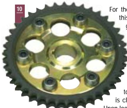
For the best possible cam timing this vernier adjustable cam gear is highly recommended, especially for competition use. Fits all models using duplex timing chain.
